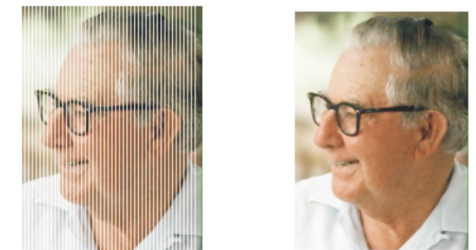
Fig. 4. Image sensor with massive column defects uncorrected (left) versus image corrected with proposed algorithm and color reconstructed (right).
