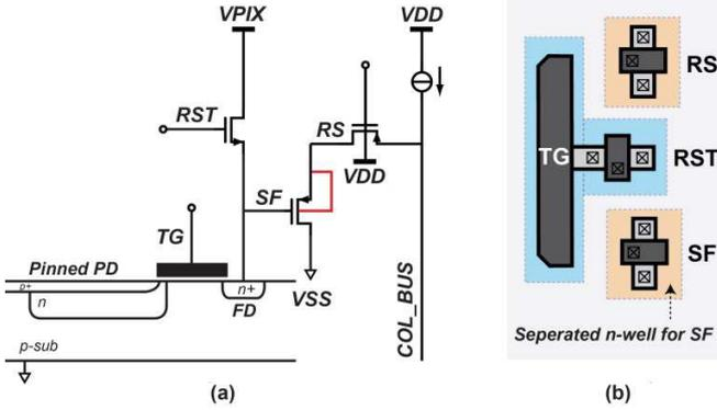
Fig. 2. Schematic of a pMOS-based SF pixel structure without body effect and the corresponding in-pixel transistors layout.
