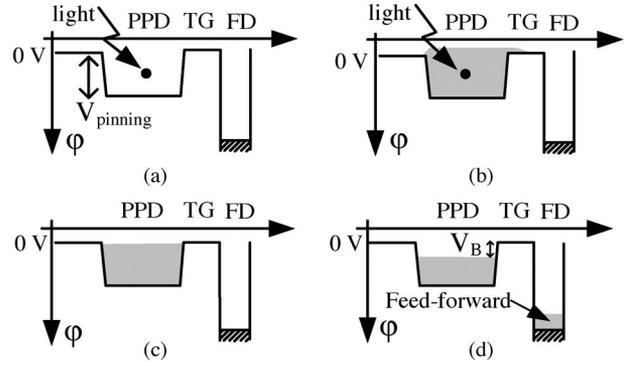
Fig. 2. PPD operation. (a) Before charge integration. (b) During and after charge integration. (c) Photodiode filled to full well. (d) Feedforward charge transfer to FD.
