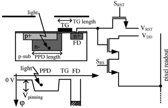
Fig. 1. Four-transistor pixel.
