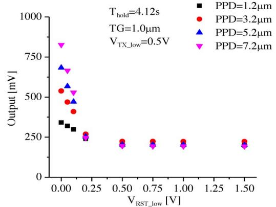
Fig. 9. FD node variation for varying  $V_{RST\_low}$  and photodiode length.
