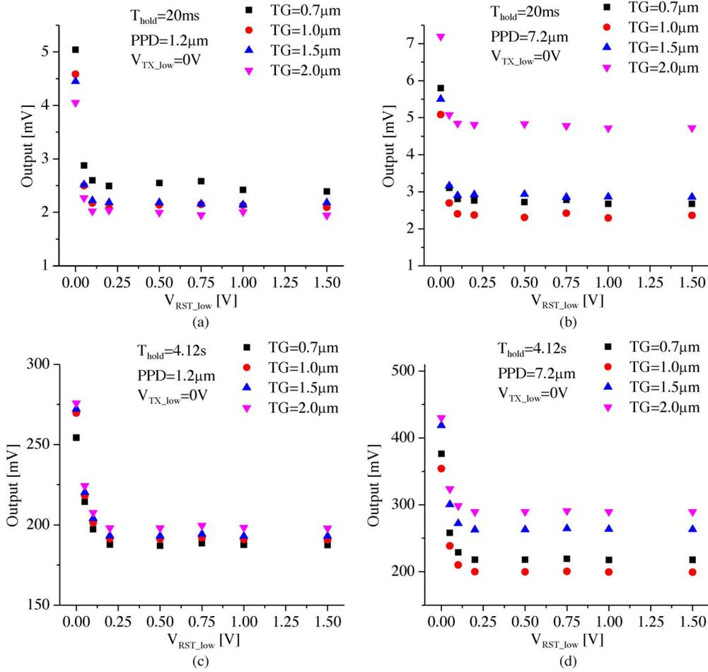
Fig. 5. FD node variation for varying  $V_{RST\_low}$  and TG lengths. (a)  $t_{hold}$  of 20 ms and PPD length of 1.2  $\mu\text{m}$ . (b)  $t_{hold}$  of 20 ms and PPD length of 7.2  $\mu\text{m}$ . (c)  $t_{hold}$  of 4.12 s and PPD length of 1.2  $\mu\text{m}$ . (d)  $t_{hold}$  of 4.12 s and PPD length of 7.2  $\mu\text{m}$ .
