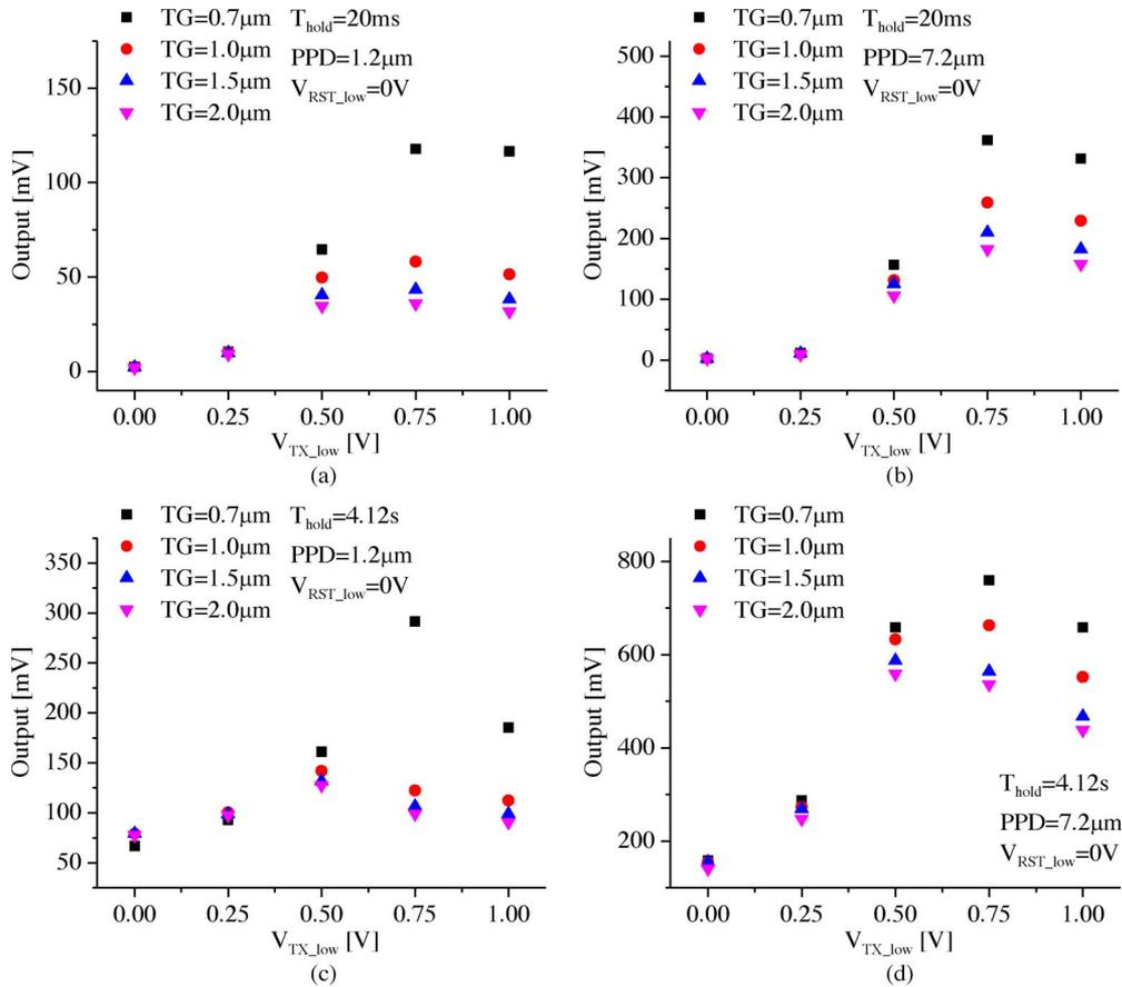
Fig. 6. FD node variation for varying  $V_{TX\_low}$  and TG lengths. (a)  $t_{hold}$  of 20 ms and PPD length of  $1.2 \mu\text{m}$ . (b)  $t_{hold}$  of 20 ms and PPD length of  $7.2 \mu\text{m}$ . (c)  $t_{hold}$  of 4.12 s and PPD length of  $1.2 \mu\text{m}$ . (d)  $t_{hold}$  of 4.12 s and PPD length of  $7.2 \mu\text{m}$ .
