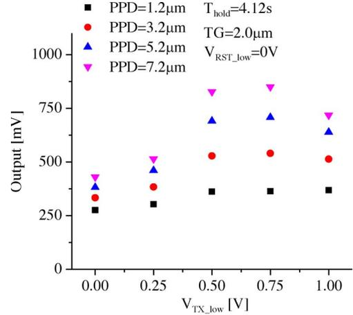
Fig. 8. FD node variation for varying  $V_{TX\_low}$  and photodiode length.
