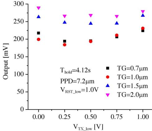
Fig. 7. FD node variation for  $t_{hold} = 4.12$  s with  $V_{RST\_low} = 1$  V.
