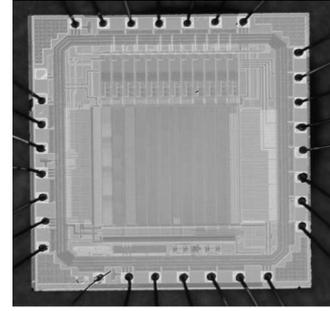
Fig. 3. Microphotograph of the test chip.
