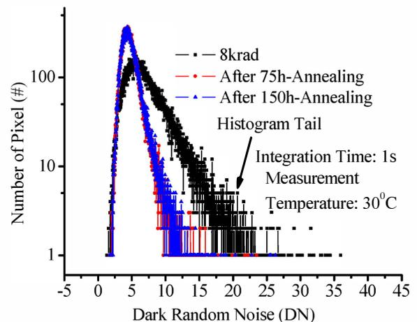
Figure 5. Annealing of the dark random noise for 75 hours and 150 hours at 85°C on an irradiated sensor.
