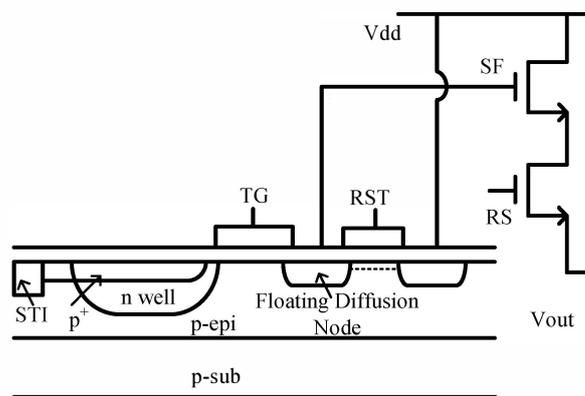
Figure 1. A 4T pixel schematic with the cross section of the PPD, the TG and the RST.
