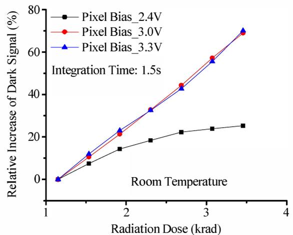
Figure 3. Pixel bias voltage effect on the relative dark signal increase with radiation doses.
