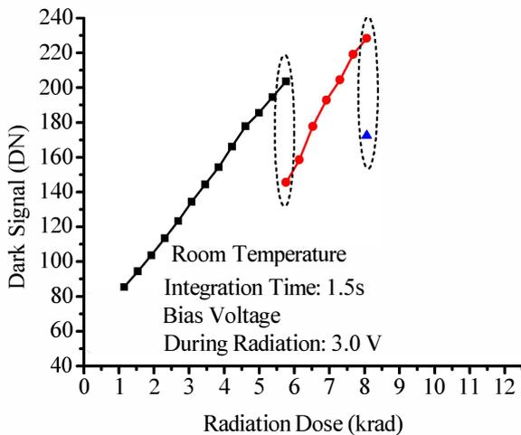
Figure 2. Dark signal versus radiation dose measured during the irradiation and 1.5 days later.
