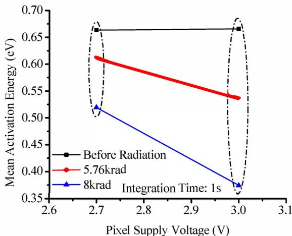
Figure 4. Mean activation energy with pixel supply voltage measured before and after radiation.
