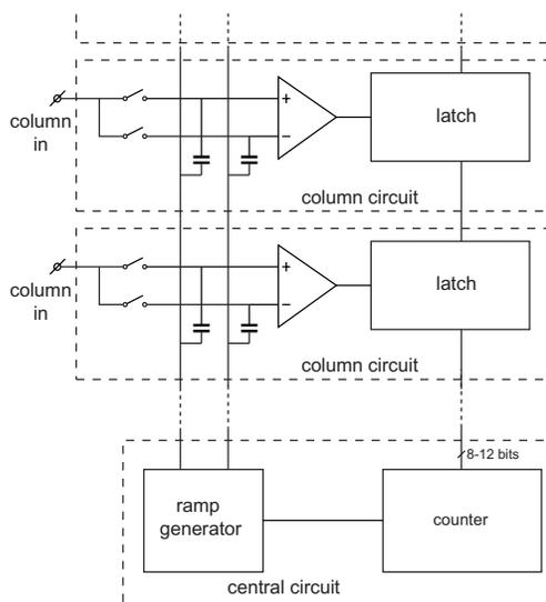
Fig. 1. Column-level single-slope ADC architecture
