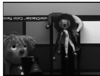
Figure 2.1.6: Vertical sub-sampling (1:6) and horizontal sub-sampling with binning (1:2) turned 'on' (1000(H)x250(V) pixels), before re-scaling (top) and after re-scaling to 4:3 aspect ratio (bottom).
