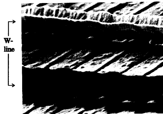
Fig. 4: SEM photograph of a deprocessed part of the storage area
